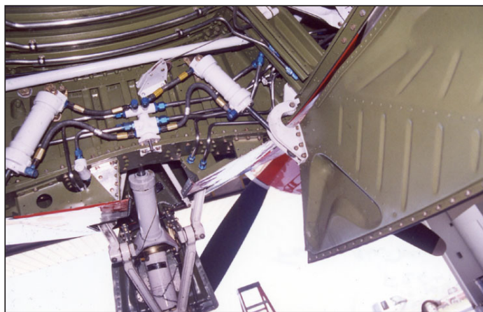
N10581 – Left main landing gear wheel well forward wall showing the well and door interiors to be green zinc chromate with white fittings. . All the sheet metal in the wheel wells are green zinc chromate.
