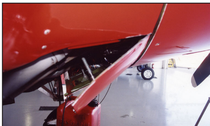
N10540 - This photograph is side view of oil cooler air outlet in the down position.
