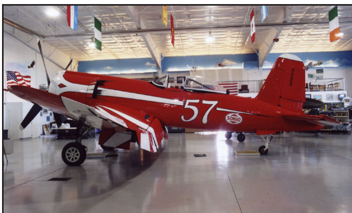
N10500 – Left side view shows the auxiliary rudder and canopy profile, which seem a little large (to accommodate the rear seat?).
