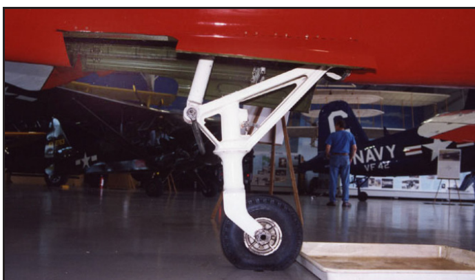
N10587 – This is the right side view of the tail wheel. It is a castoring wheel and is swiveled as a result of the plane being pushed back into position.
