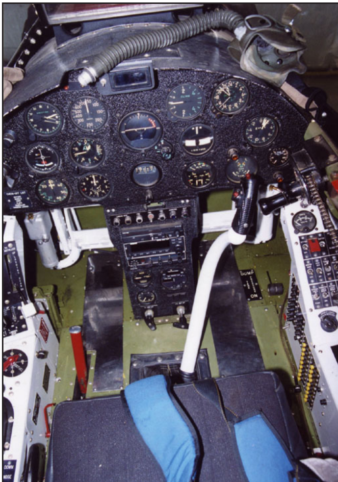
N10505 – Looking down and forward in the cockpit you can see the rudder pedals are white and the heel rub strips are polished metal.
