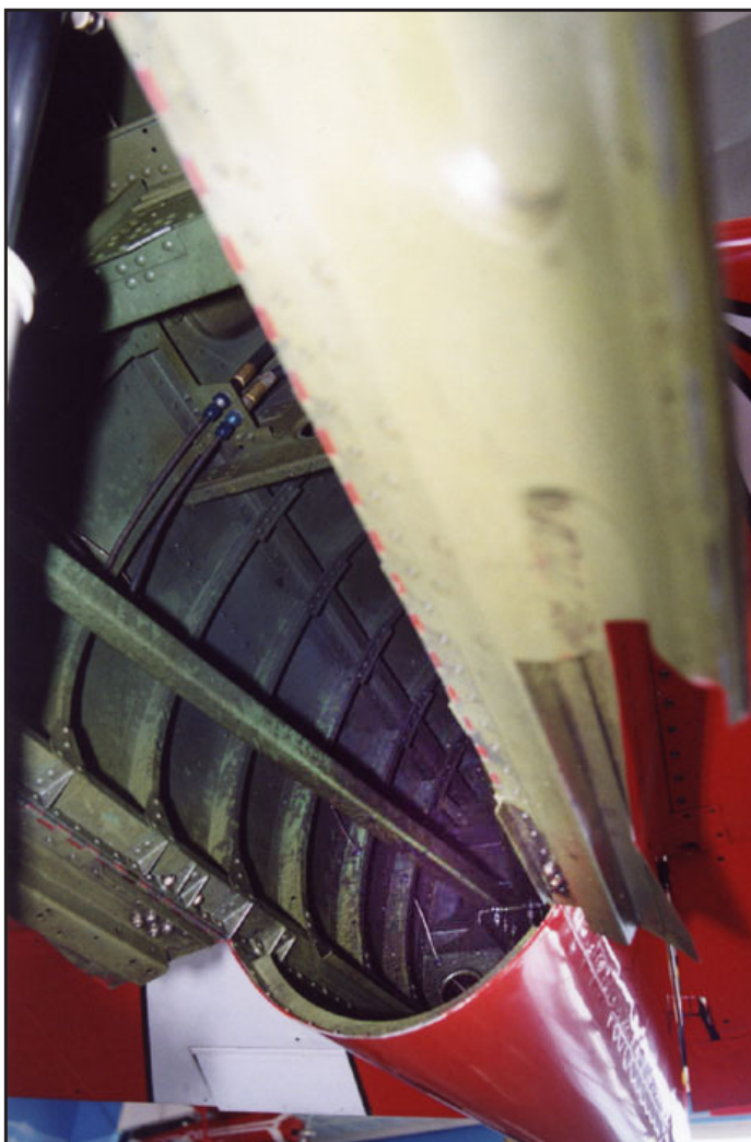
N10592- This aft view of the tail wheel well shows the interior of the well and tail wheel gear covers to be green zinc chromate.
