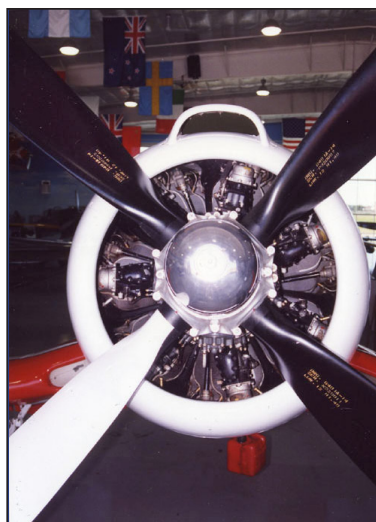
N10567 – Front view of the engine and propeller hub. Note that you really cannot see the second row of cylinders due to the ducting directing air to the rear cylinder banks.
