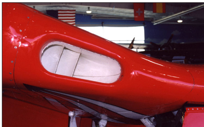
N10544 - The left wing oil cooler inlet is a mirror image of the right wing inlet.
