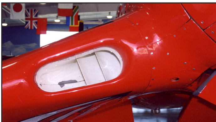
N10542 – The right wing oil cooler air inlet is different than the F4U. The radiators are in the fuselage on the F2G while they are in the wings on the F4U. This view shows the inlet guide vanes ducting the air inboard.
