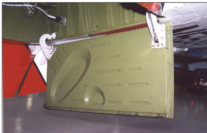
N10584 – Left main landing gear wheel well outboard door interior.
