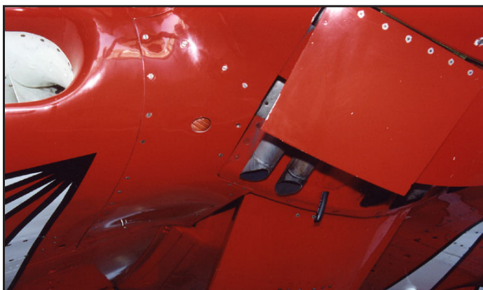
N10541 – This photograph shows the lower exhaust pipes and the oil cooler air outlet in the down position.
