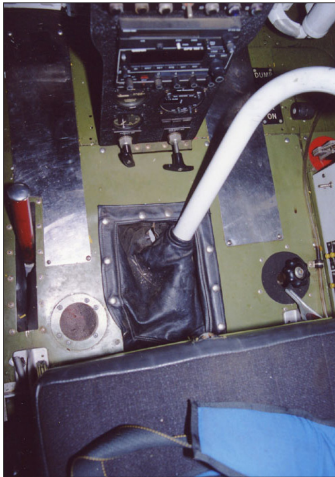
N10526 – Cockpit floor details with the control column boot in black leather or leatherette.
