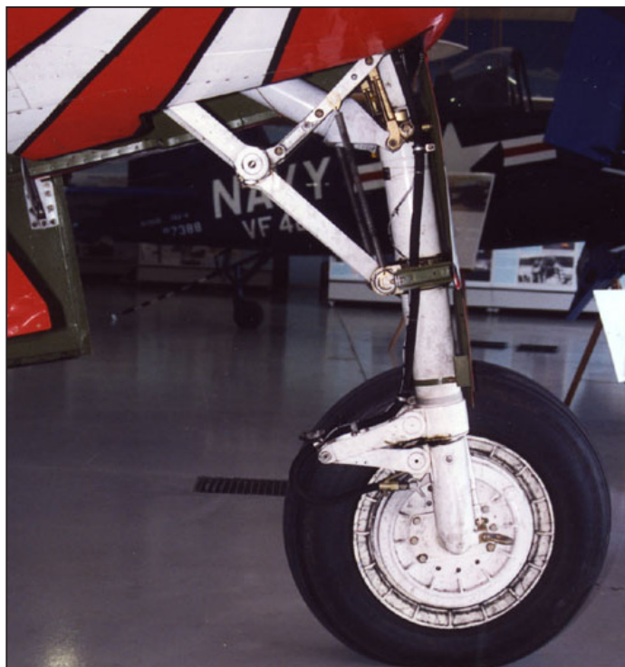
N10573 – Inboard view of the left main landing gear.
